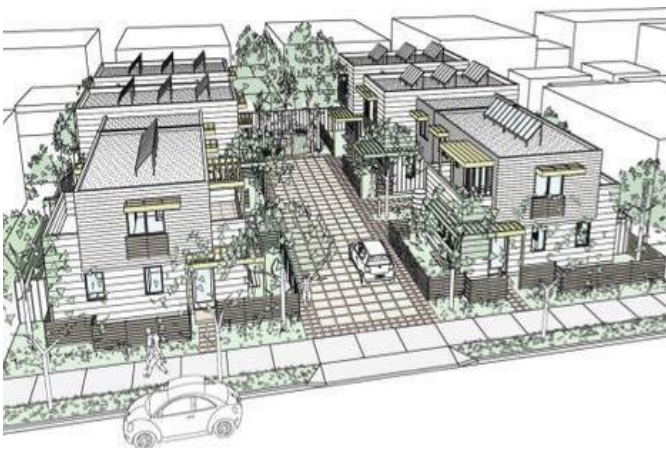
Illustrates courtyard ownership or rental housing with units clustered on a property around shared open spaces and amenities,
