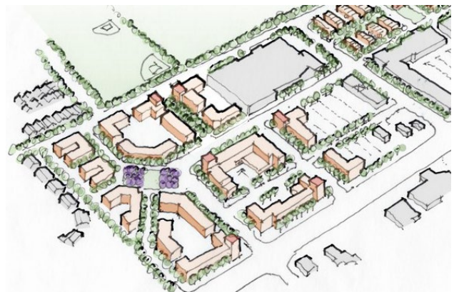
Illustrates revitalized development of the Mission Bell Plaza site by retention of existing buildings (shown in gray) replacement of others, and construction of new buildings on surface parking lots (color highlighted). Buildings contain a mix of retail and housing, front onto, and are oriented to new internal street grid with pedestrian-oriented amenities. Parking is consolidated in structures.
