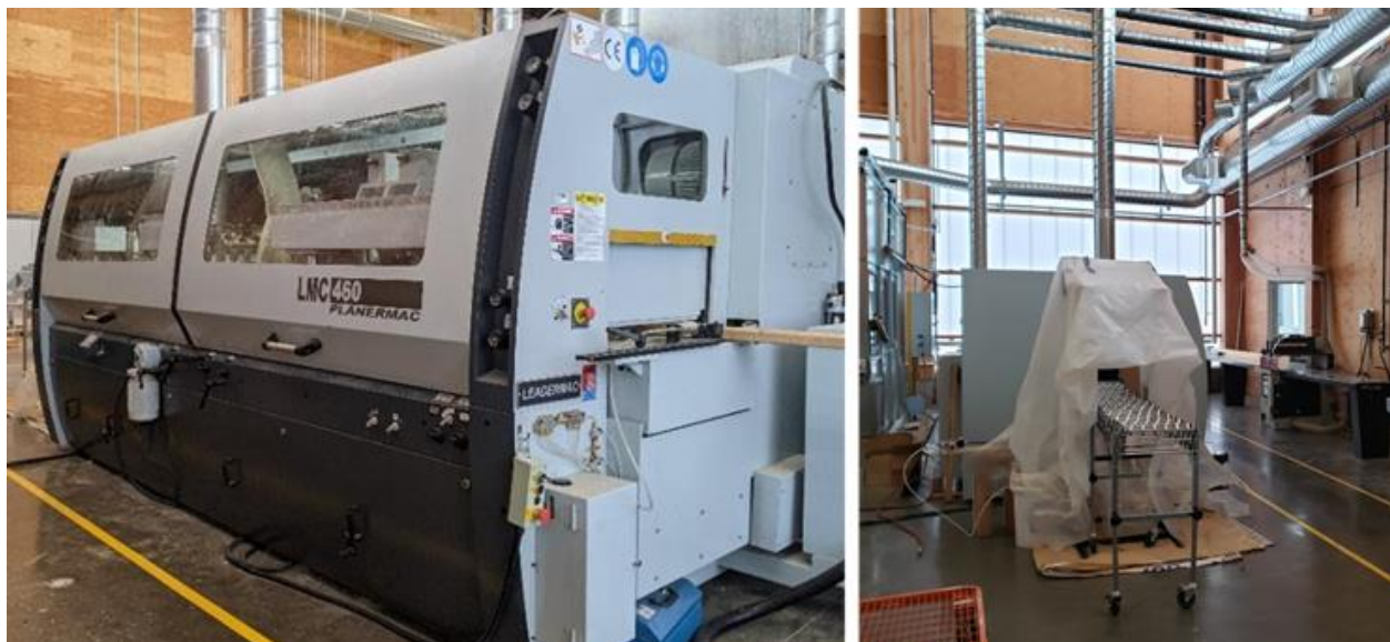
Figure 3: Leadermac Planer (left) and primer setup connected to the outfeed of Planer (right)
