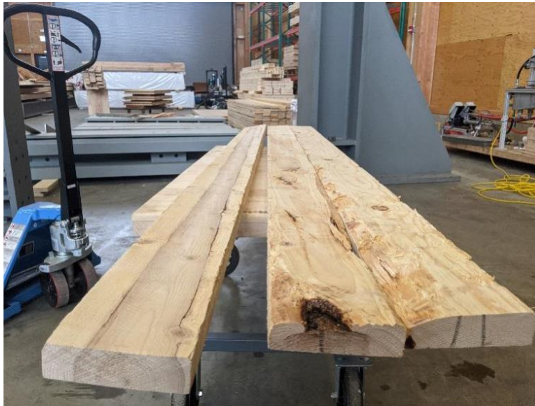
Figure 1: Examples of rejected boards
