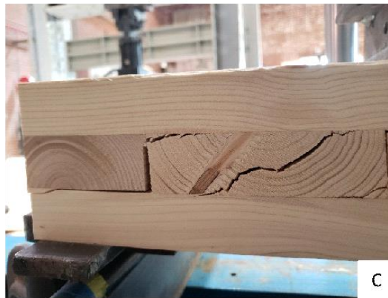
Figure 14: (A) and (B) short span testing setup side and top view, respectively. (C) Typical sample failure, failing in shear
