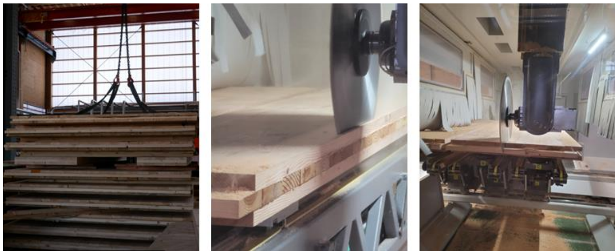
Figure 8: (Left) CNC panels about to be lifted into CNC, (Center) CNC performing ripping operation on panels, and (Right) CNC performing cross-cutting of panels
