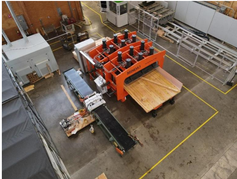
Figure 6: Appiqu resin applicator and Minda press
