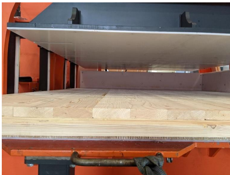
Figure 7: CLT panel immediately after pressing
