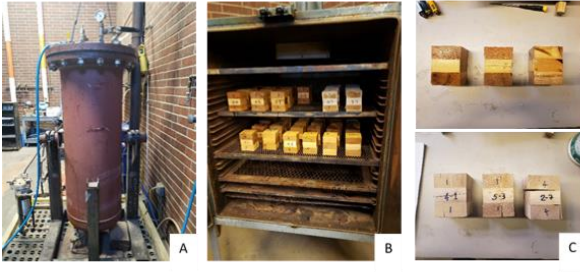
Figure 12: (a) Vacuum/Pressure Vessel, (b) Air Circulating Oven with Samples, and (c) Top: Samples after soaking, Bottom: Samples after drying
