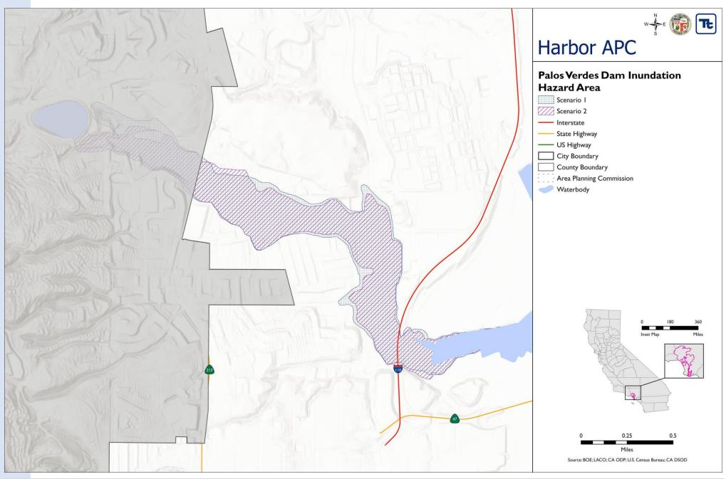
Figure 8-11. Palos Verdes Dam Failure Inundation Area
