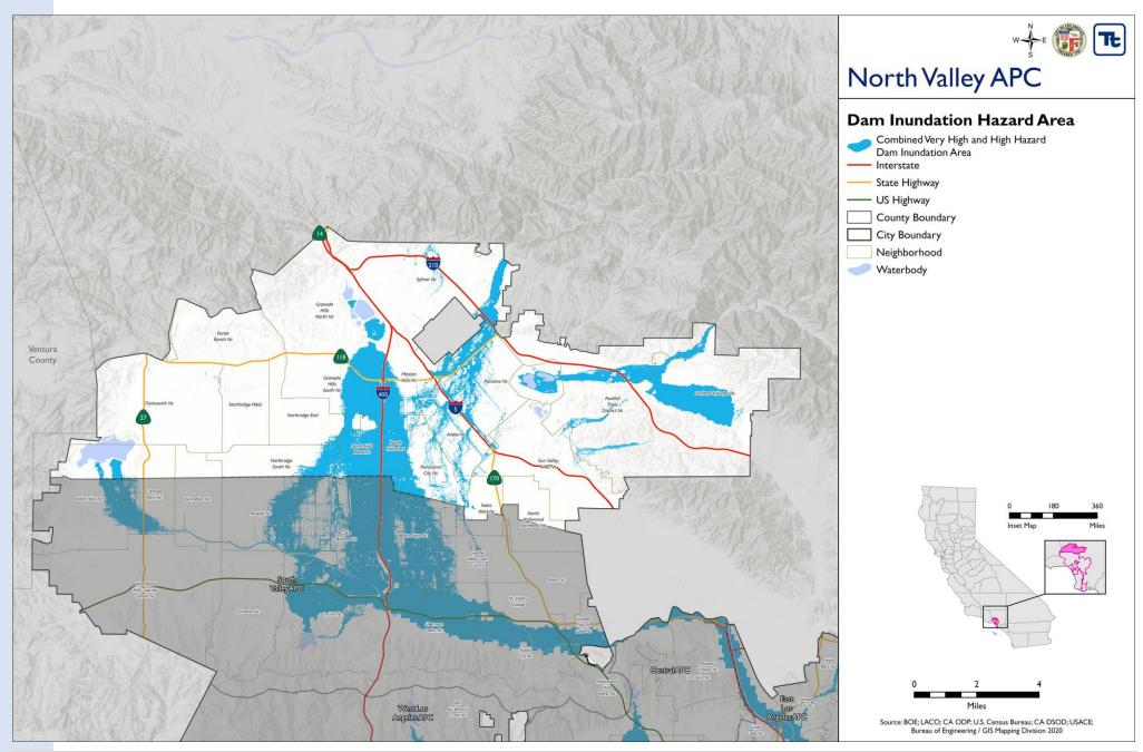
Figure 8-2. North Valley APC Combined Dam Failure Inundation Area
