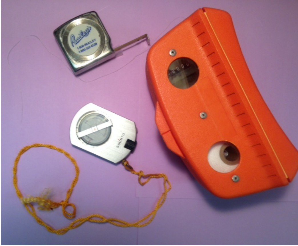
Figure 25. The tools needed to complete road monitoring included (1) pocket tape measure (erosion void dimensions), (2) string box (distances), and 3) clinometer (gradients). Also needed were the FORPRIEM road forms and a digital camera (optional).
