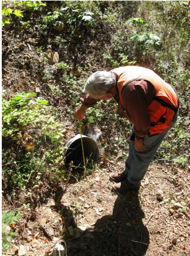
Figure 54. Clay Brandow measuring the pipe diameter on a FORPRIEM THP located in the upper Sacramento River Canyon.
