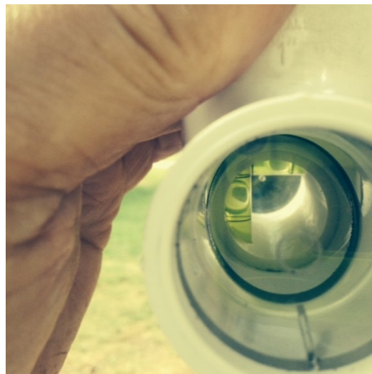
Figure 10. Standard procedures for use of the sighting tube included bringing the instrument up to the observer's eye, centering the two leveling bubbles, moving the observer's head slightly to center the dot in the circle, determining if canopy exists above the instrument, and recording a hit or miss on the data form.
