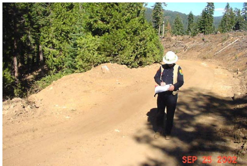
Figure 6. Pete Cafferata recording road observations at a rolling dip. Orange box on his right hip is a hip-chain which meters-out string for tracking distances of specific road-related features along the sample segment.
