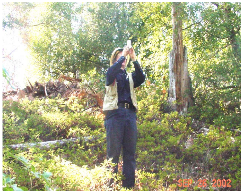
Figure 1. Pete Cafferata making WLPZ canopy cover measurements using a sighting tube.
