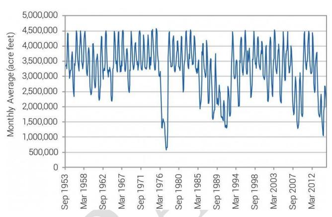
Figure 4.8 Storage Levels in the Shasta Dam Reservoir
