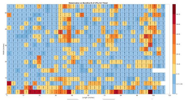
Figure 10. Color coded *Delamination map* for two bond planes in 3-ply MF panel. Color scale reflects the percent of delamination in each block measured after PRG320-2019 PRG delamination test (shades of blue show acceptable level of delamination or pass).
