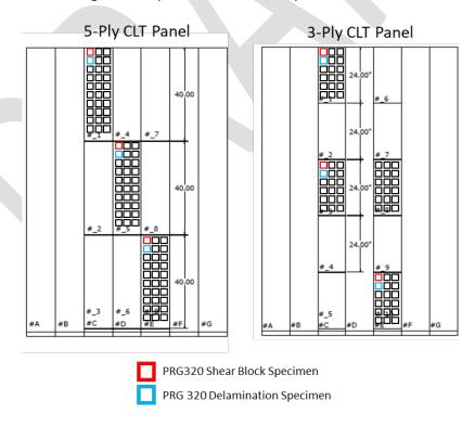
Figure 5: PRG320-2019 subsample locations for shear block and cyclic delamination specimens
