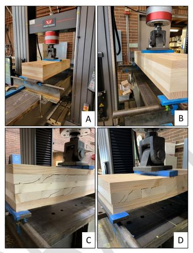
Figure 7: (A&B) Short-Span Shear Test Setup, (C) 5-ply shear failure, (D) 3-ply shear failure
