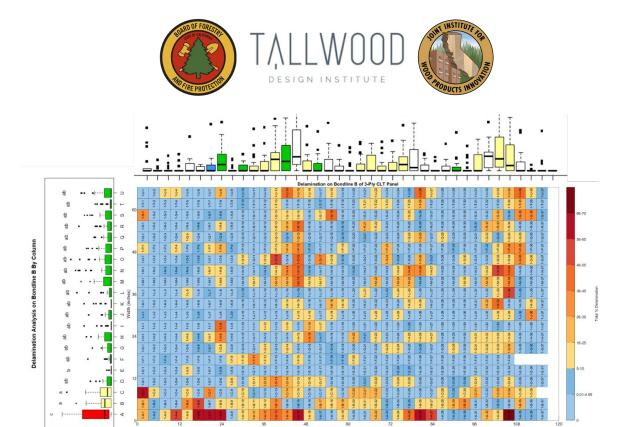
Figure 15. Distribution of frequency of delaminations within individual bond planes in 3-ply MF panels within horizontal and vertical strips. Alignment along individual laminations may be an indication of an effect of lamination thickness variation
