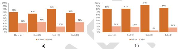
Figure 13. Comparison of proportions of specimens passing and failing the PRG320-2019 delamination tests in 3-ply (a) and 5-oly (b) MF panels by categories: clear specimens (A), specimens with knots touching a bond plane (B), specimens with inter-lamination gaps (C) and with both, knots and gaps (D). (Based on n=775 in both panels).
