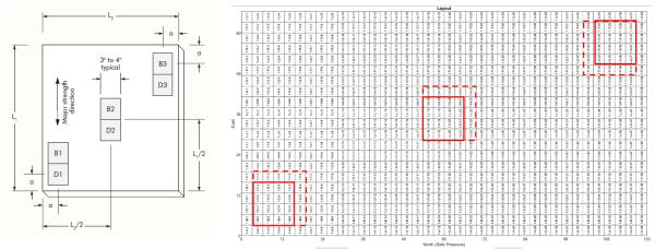
Figure 8. Standard PRG320 sampling scheme for delamination specimens allows more options in small lab-scale billets (left) than in larger test panels (right).
