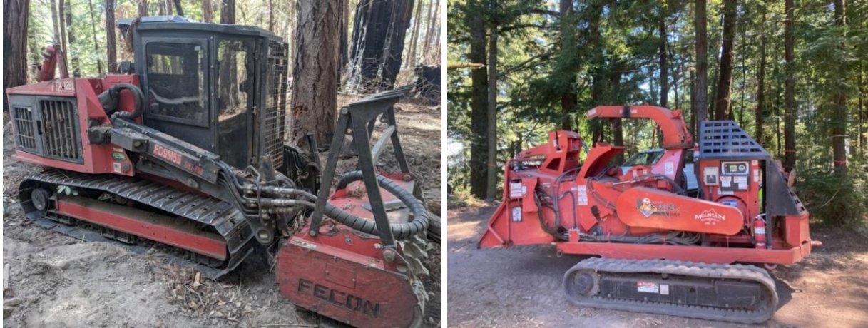
Figure 15. Examples of Mechanized Equipment – Fecon FTX 128 Series compact track loader with masticating head attachment (left). Morbark Beaver M15R tracked chipper (right)
