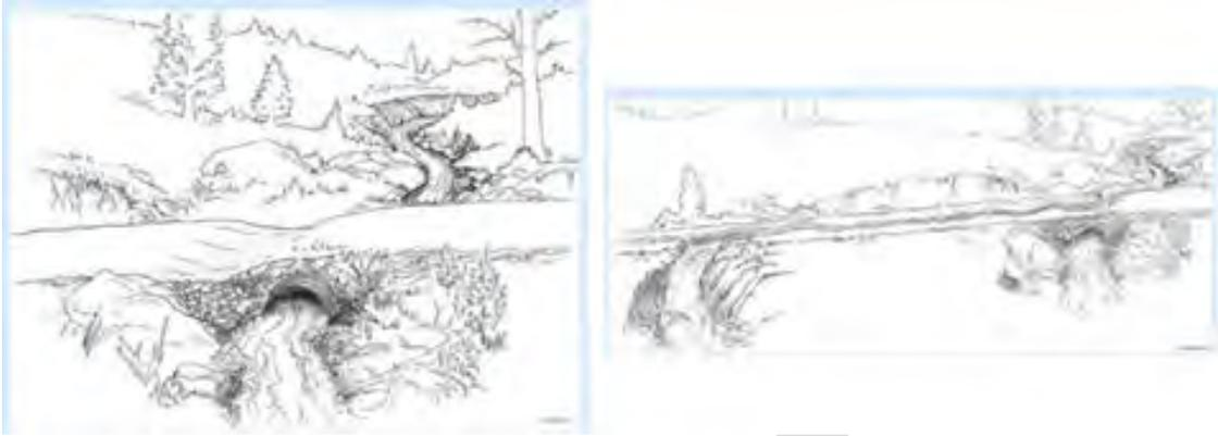
Figure 5: No potential for diversion (Left), and potential for diversion (Right) (Images from Furnis et al., 1997)
